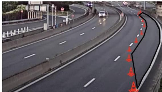
*Figure 8 Polygons are drawn on the device screen to designate the area that needs to be monitored for intrusions*
